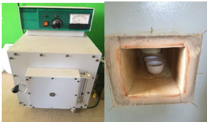
Figure 3 Testing of combustion properties of samples in muffle furnace
